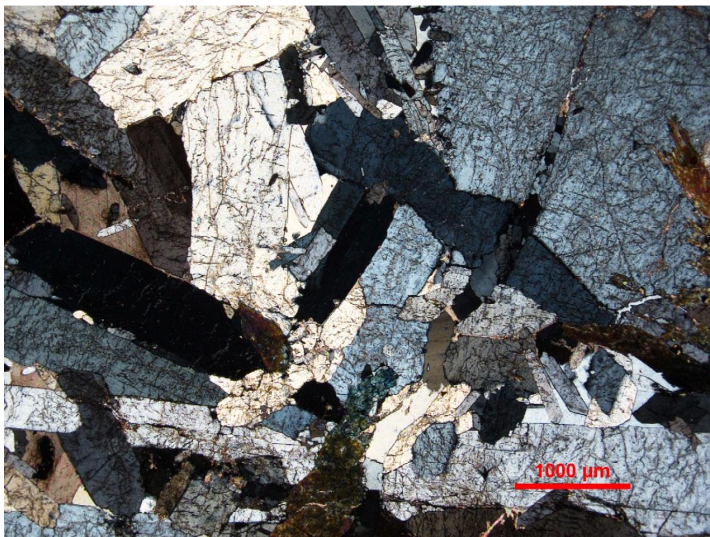
Sample 863669. Coarse, subhedral, elongated axinite(?) grains with strong internal fracturing. Top- plane light; Bottom- crossed polarizers.
