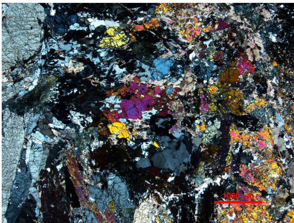
Sample 863669. Main band of epidote-tourmaline-carbonate-quartz alteration cutting axinite. Top- plane light; Bottom- crossed polarizers.
